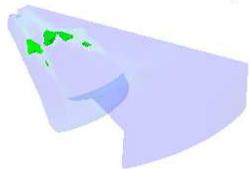
CO2 Mass Fraction of Diesel (Above) and H2 HPDI (Below)
