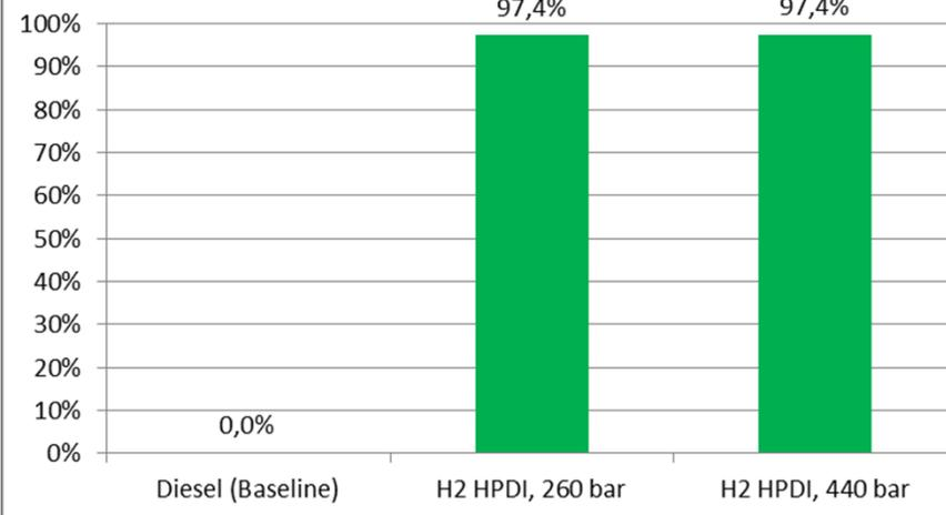
CO2 reduction of 97.4% from diesel baseline at the high load point with H2 HPDI
