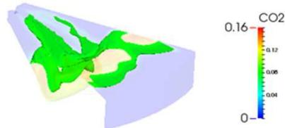
CO2 Field During Hydrogen HPDI Combustion Showing 94.8% Reduction of CO2 Compared to Diesel
